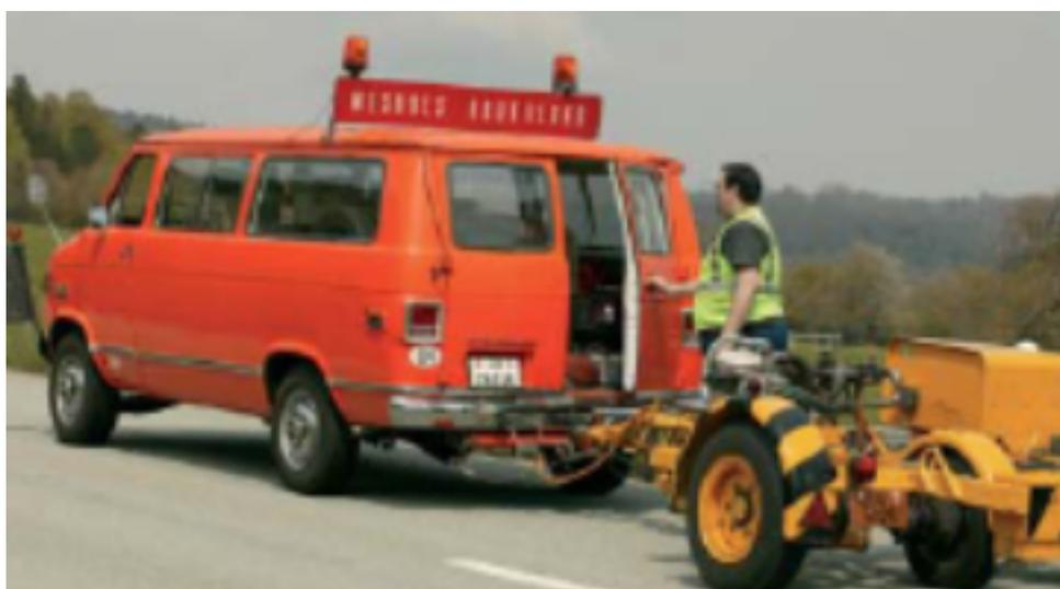
Figure 3 - Skiddometer BV11
